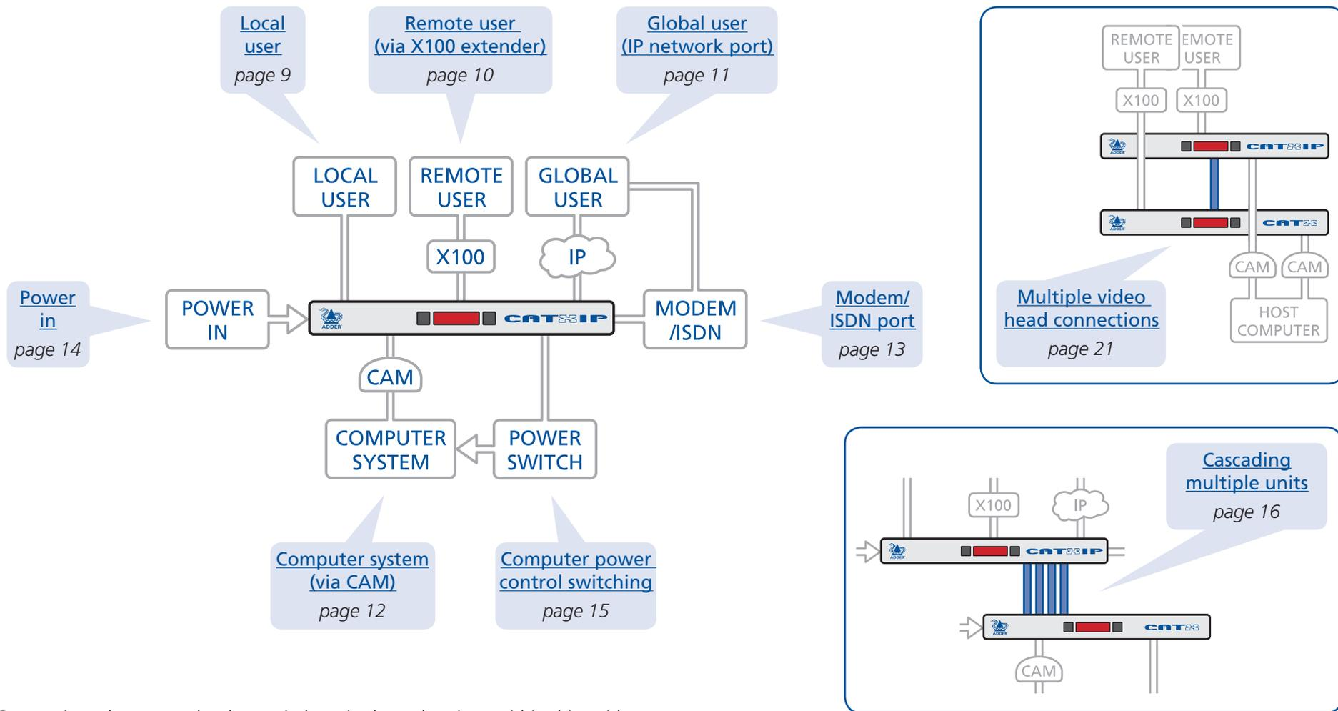
Connections do not need to be carried out in the order given within this guide, however, where possible connect the *power in* as a final step.
