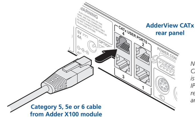
Note: The AdderView CATx model shown here is a non-IP version. The IP-version provides only remote user ports 3 and 4.
