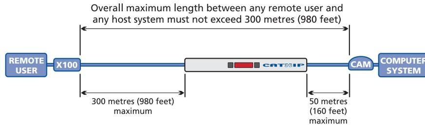
In situations where any computer system will be placed a significant distance from the AdderView CATx unit, ensure that the distance to any remote user is similarly less than 300 metres (980 feet).
