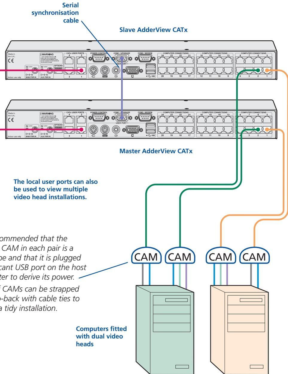
The local user ports can also be used to view multiple video head installations.
