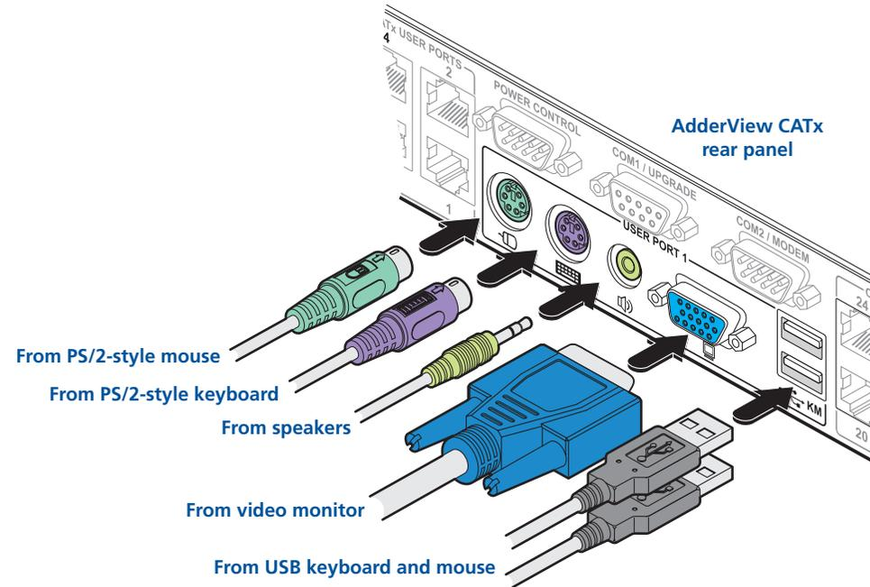
*Note: The keyboard and mouse can be either PS/2-style or USB respectively, as required. The two different connection types can even be mixed. Recognition of the type used is automatic and requires no extra settings to be made.*
