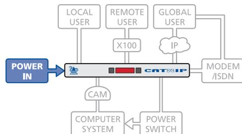
*Note: AdderView CATx units require a heavy duty power adapter at either or both power input connectors. Use only the adapter supplied with the unit or available under Adder part numbers: PSU-IEC-5V4A (for AdderView CATx) or PSU-IEC-5V6A (for AdderView CATx IP). Do not use the standard 10W adapters that are supplied with other Adder products, such as the X100.*
