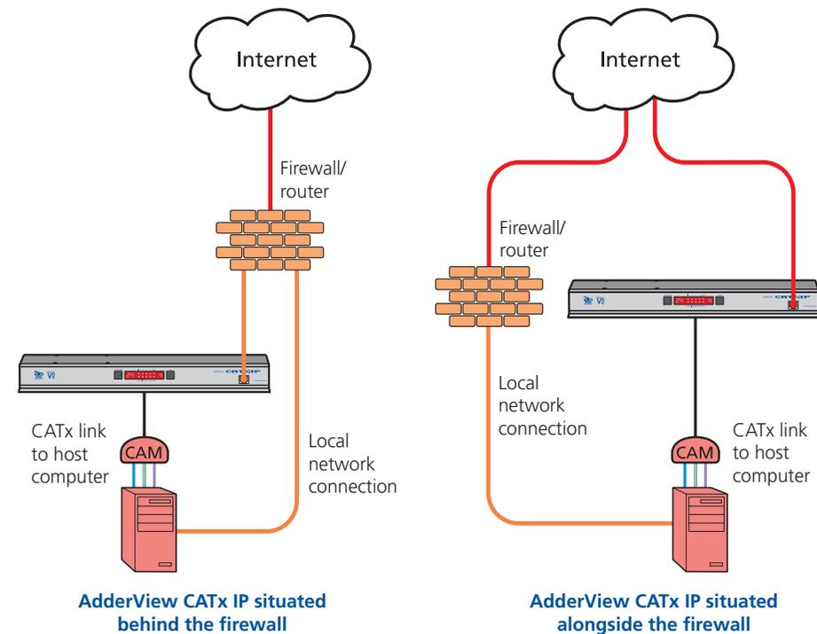
*IMPORTANT: When the AdderView CATx IP is accessible from the public Internet or dial up connection, you must ensure that sufficient [security measures](#) are employed.*
