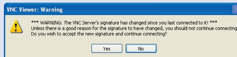
This message is displayed if an AdderView CATx IP unit, that your viewer has previously visited, has had a change of security keys. This is not uncommon if a unit is reset for some reason. However, it could also mean that your trusted unit is being spoofed and you may not be connecting to the system that you think you are.
