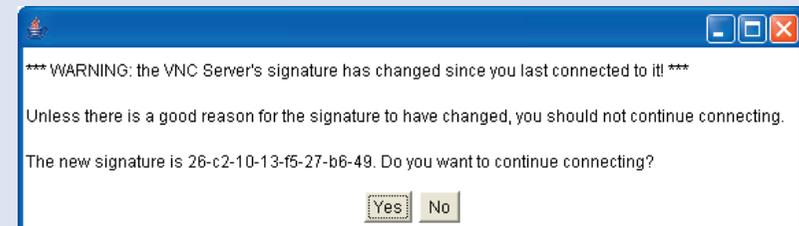
This message is displayed if an AdderView CATx IP unit, that your viewer has previously visited, has had a change of security keys. This is not uncommon if a unit is reset for some reason. However, it could also mean that your trusted unit is being spoofed and you may not be connecting to the system that you think you are.
