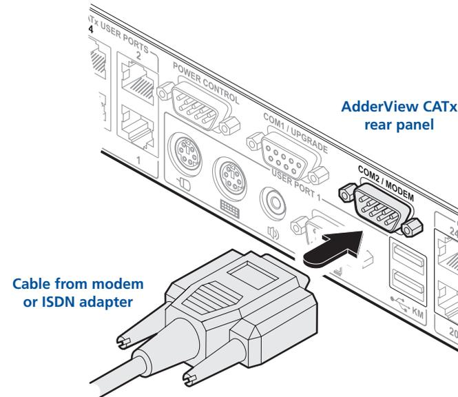
*Note: The default serial port speed is 115200 and a standard Hayes-compatible auto-answer string is sent during startup. The default startup string is 'ATZHS0=1'. Both the serial port speed and startup string settings can easily be altered during configuration - see [Initial IP configuration](#) for more details. The other serial settings are fixed at: No parity, 8 bit word and 1 stop bit.*
