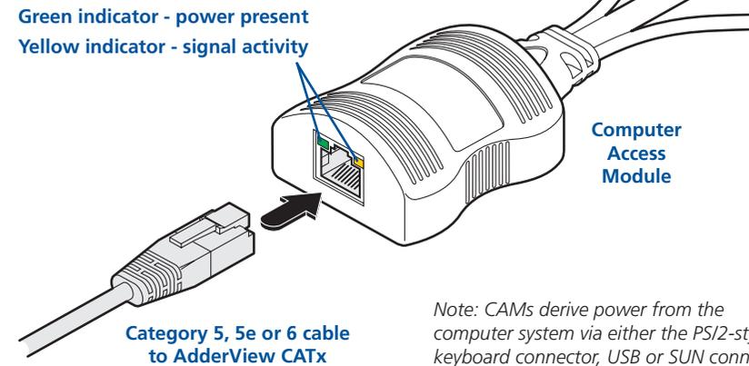
*Note: CAMs derive power from the computer system via either the PS/2-style keyboard connector, USB or SUN connector.*
