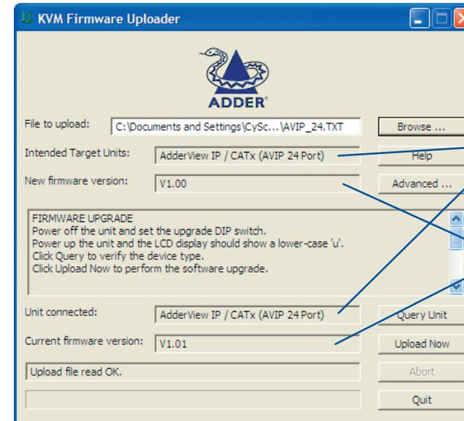
Check that the 'Intended Target Units' field matches the 'Unit Connected' field.
