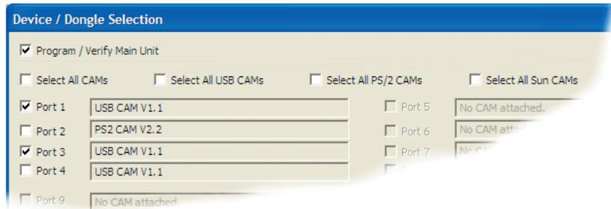
The type and firmware revision of each discovered CAM will be displayed alongside the port number to which it is connected.
