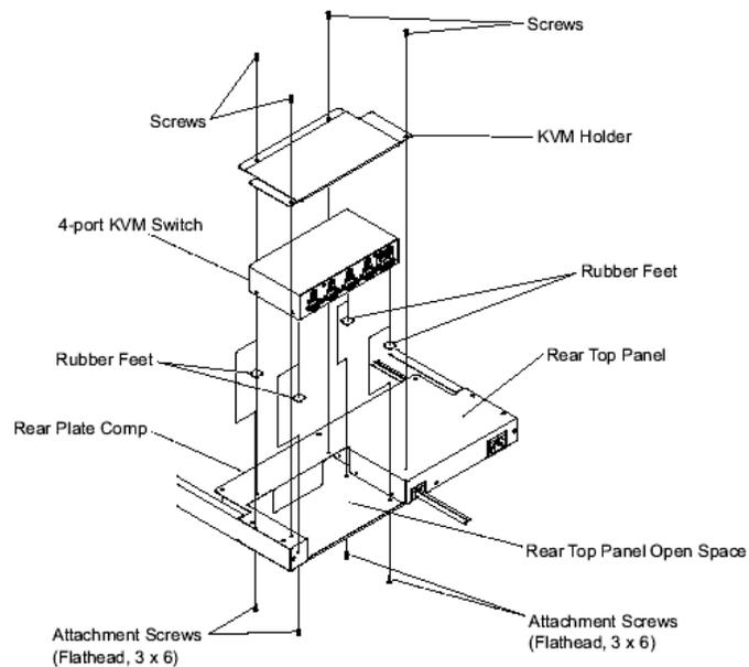
Installation Method 2: 4-port KVM switch Assembly Diagram
