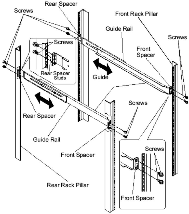
Installing the Guide Rails diagram
