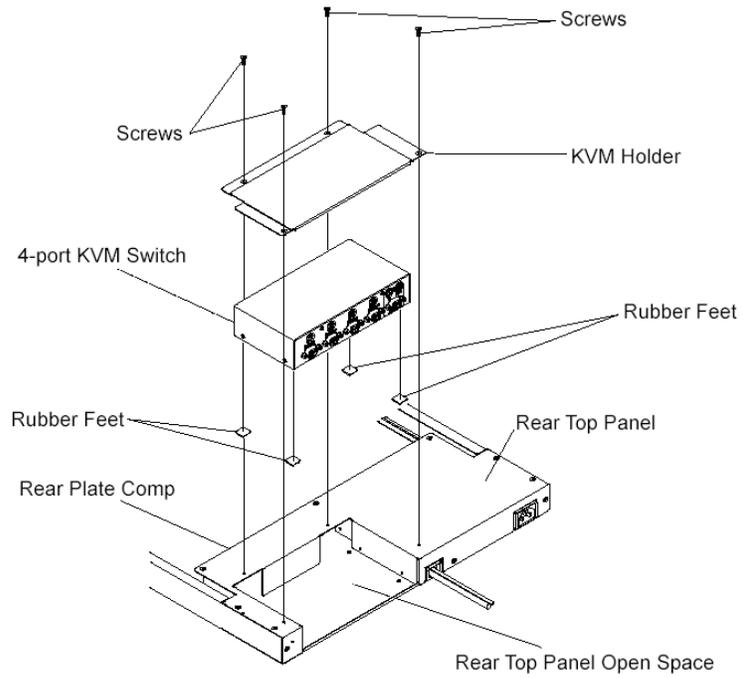
Installation Method 1: 4-port KVM switch Assembly Diagram
