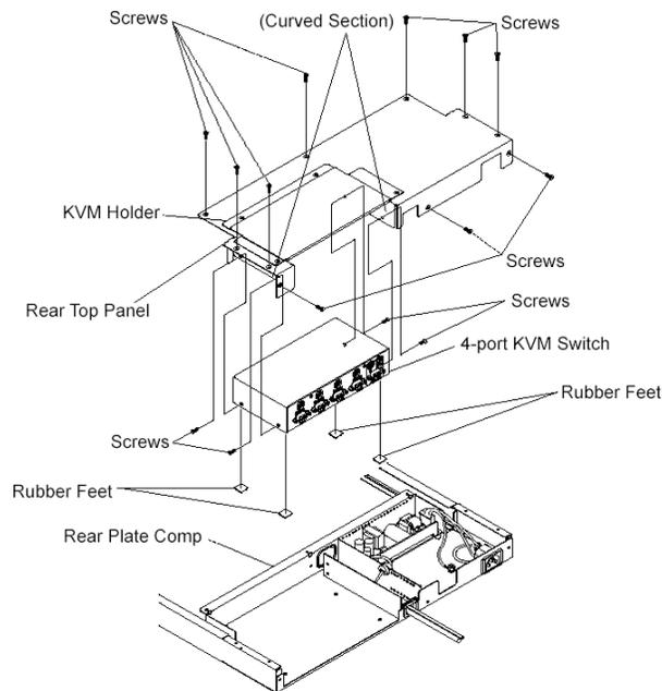
Installation Method 3: 4-port KVM switch Assembly Diagram
