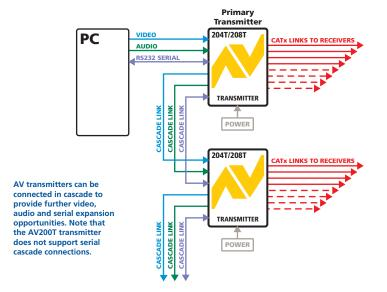
Note: The AV200T transmitter supports video and audio cascade connections, however, the module does not include a serial out connector and cannot support cascaded serial connections.
