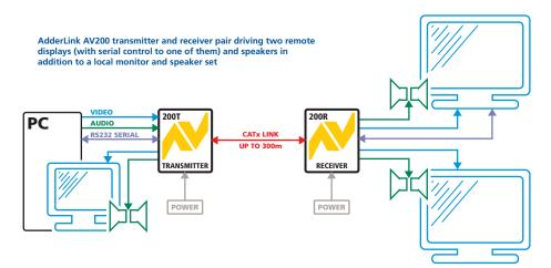
The AV200P transmitter and receiver modules are also available separately and are known as the AV200T and AV200R respectively. Expansion is made possible by connecting further transmitters to the original AV200T transmitter module, however, the serial connection cannot be cascaded in this manner. Where cascades with serial connections (as well as video and audio) are required, use the AV204T/AV208T transmitters
