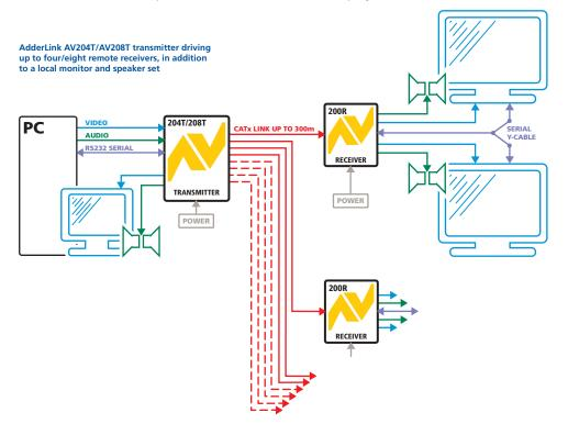
Additional expansion is also possible by connecting further transmitter modules to the original module in a cascade arrangement, each supporting their own multiple AV200R/AV201R receiver modules - See *Expansion via cascade links* for details.
