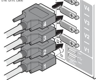
Note: On the rear panel of the unit, connectors belonging to the same channel are stacked vertically. The connectors at each horizontal level (V1 to V4) will be switched through to the user console DVI-I connector which is at the same level:
