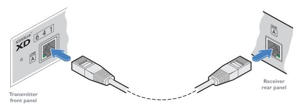
2 In operation, ensure that both indicators on the CATx connectors are green. See right.
