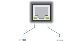
This indicator will be green whenever there is a CATx link between the transmitter and receiver modules.
