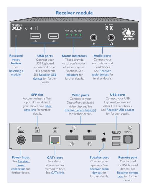
The transmitter and receiver modules are contained within slimline metal casings that measure just  $186 \times 152 \times 40$ mm.
