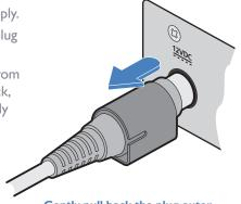
Gently pull back the plug outer body to release the lock
