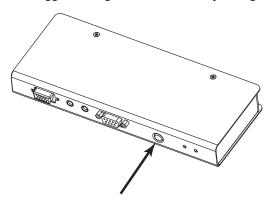
**Note:** Remote mode cannot be selected. The remote console can get control only when the Operating Mode Pushbutton on the CE750AL is toggled to *Auto* and the local console is idle. If the remote console is then idle for more than five seconds, the local console can gain access.
