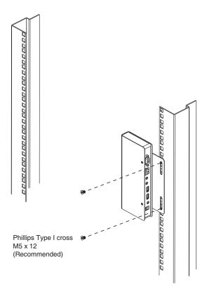
**Note:** These screws are not provided. We recommend that you use M5 x 12 Phillips Type I cross, recessed type screws.
