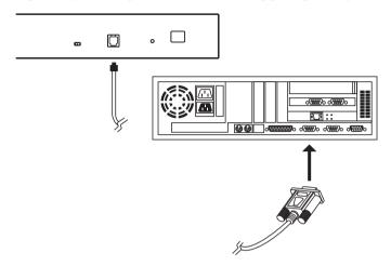
**Note:** On a daisy chained installation, connect the cable to the first station (master) unit. The chained stations (slaves) that are the same model will receive the upgrade via the daisy chain cables.
