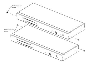
2. Screw the mounting brackets into the sides of the unit at the front or the rear, as shown in the diagram below.
