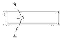
2. Make sure the computer that the Transmitter connects to and the monitor that the Receiver connects to are properly grounded.
