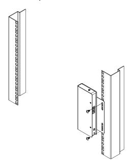
**Note:** These screws are not provided. We recommend that you use M5 x 12 Phillips Type I cross, recessed type screws.
