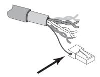
b) The second method is to use the STP cable shielding for grounding. In this case, make sure that the shielding makes tight contact with the top inside of the RJ-45 connector as shown in the diagram below:
