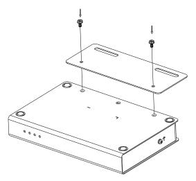
3. Screw the bracket into any convenient location on the rack.
