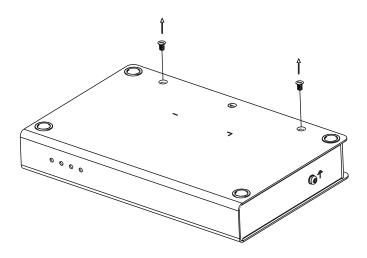
2. Using the screws provided in the Mounting Kit, screw the mounting bracket on to the bottom of the unit as show in the diagram, below:
