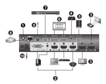
1. Use a grounding wire to ground the unit by connecting one end to the grounding terminal, and the other end to a suitable grounded object.
