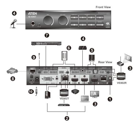
Use a grounding wire to ground the unit by connecting one end to the grounding terminal, and the other end to a suitable grounded object.
