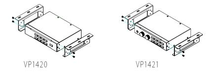
Position the unit to a spot under the desk where you can easily access the front panel, and then secure the racks to the desk with self-prepared screws.
