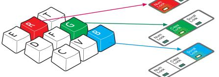
5 Press the  $\boxdot$  and  $\boxdot$  keys to retard or advance the timing of the selected colour channel respectively. On screen you will see a change in the position of the selected colour crosses in relation to the other two.
