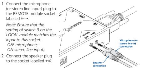
Note: When the X2-Gold REMOTE module is rack mounted, the audio connections must be made after the module has been fixed in place. Access is required to the rear and above the rack. Remember to remove the audio connections before attempting to slide out the REMOTE module. Ò 0 D  $\bigcirc$  $\bigcirc$
