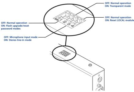
Note: When shipped, all switches are set in the OFF positions and this will produce normal operation with normal microphone input (at the REMOTE module).
