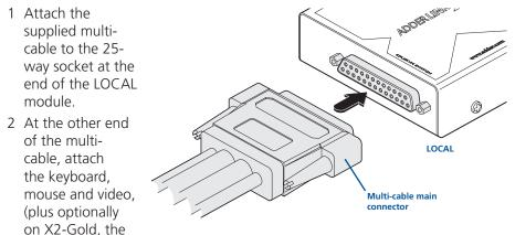
microphone and speaker) connectors to the appropriate sockets at the rear of the computer system. On most systems the appropriate ports should be labelled and colour coded in a similar way to the cable connectors:
